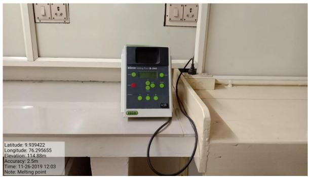
Melting Point Apparatus is used to measure the melting point of compounds separated by qualitative analysis
