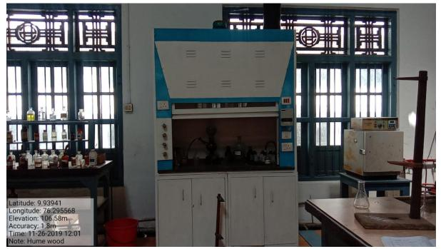
Fume hoods are used to do experiments and protect the students by Containing vapours, dusts, gases, and fumes generated within the **hood**, and removing them as air flows into the **hood** and then out via the laboratory exhaust system.
