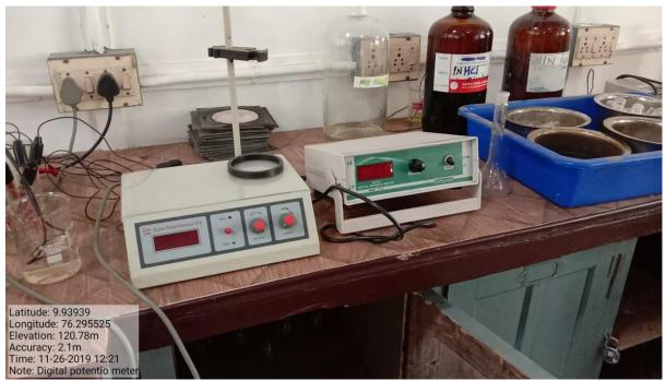
The measuring instrument called a **potentiometer** is essentially a voltage divider used for measuring electric potential (voltage) This apparatus is used to conduct physical chemistry experiments. It is used to measure the EMF of solutions and in potentiometric titrations and measuring the solubility of substances .
