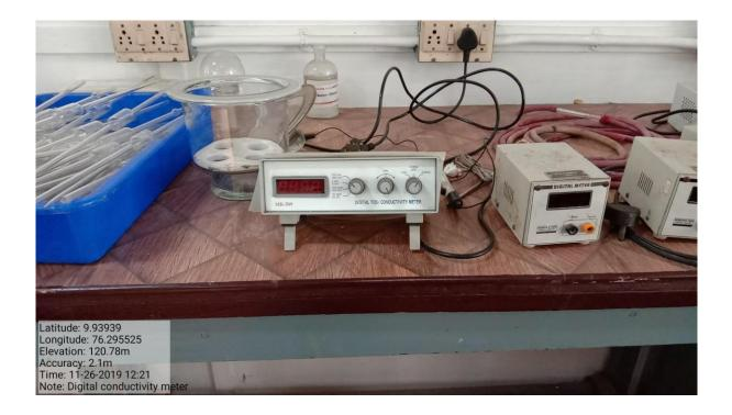
A digital conductivity meter accurately measures the amount of electrical current or conductance in a solution. Conductivity meter is used in conductometric titrations in physical chemistry experiments.
