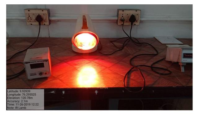
In science the I.R lamp is mainly used for heating. It is used to dry the compound prepared during organic and inorganic synthesis experiments. Use:- in drying the compounds.
