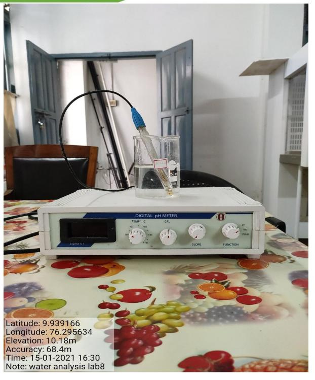
Digital pH Meter is an important instrument for determining the pH of the solutions ie. the acidity or alkalinity of the samples can be determined. It consists of a voltmeter and a glass electrode. The electrode is dipped in the solution in which the pH is to be determined and we get the voltage proportional to the H ion concentration.
