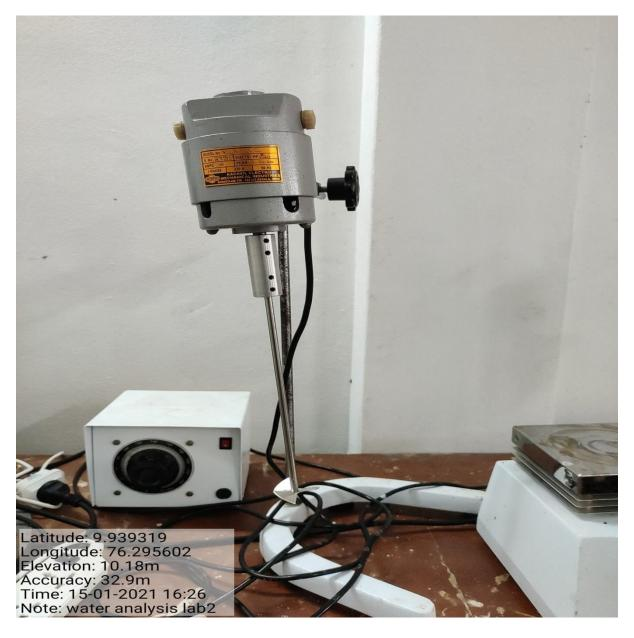
Mechanical stirrer is a vertical stirrer with a working motor used for the mixing and stirring of different samples. It allows the mixing of different liquids and suspensions by immersing the vertical rod in the sample thus the stirrer blend the samples well and make the reaction faster.
