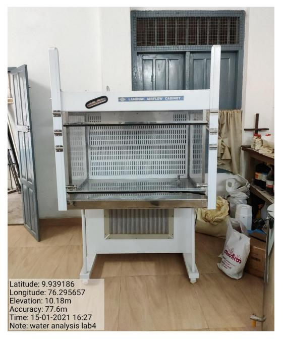
Laminar airflow cabinet is an enclosed bench used for the safety of different samples especially biological samples and sensitive materials. It is made up of stainless steel and due to the laminar air flow sample can be kept safe. The UV lamp and FL lamp within the instrument sterilize the samples.
