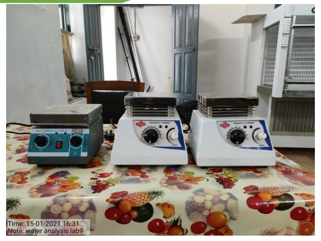
Magnetic stirrer is an instrument used for stirring of samples in presence of magnetic field. It consists of a hot plate and magnets within the instrument. It can be used for the even mixing of samples which is kept at the hot plate along with a magnetic rod. The speed and temperature can be adjusted.
