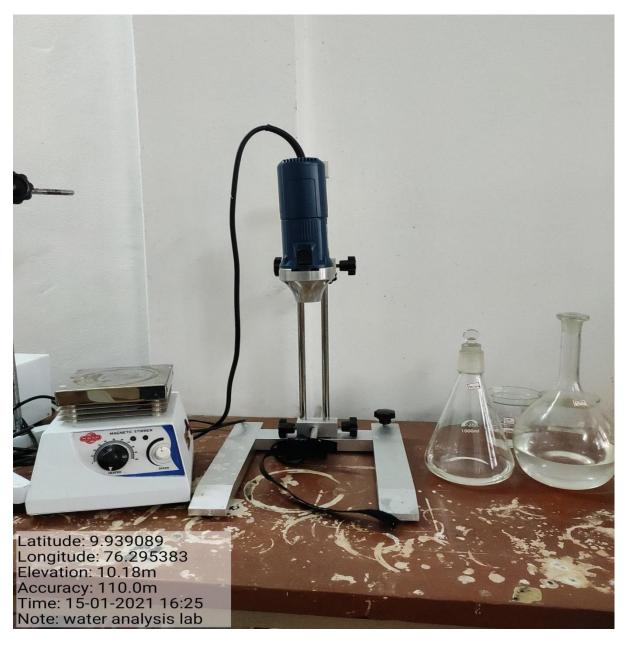
Homogeniser consists of a working motor and a long probe. It is used for the reduction of size of the samples usually dispersions or liquid samples to obtain a solution with uniform distribution and composition. The energy passing through the liquid applies a force and shears the substance to smaller size.
