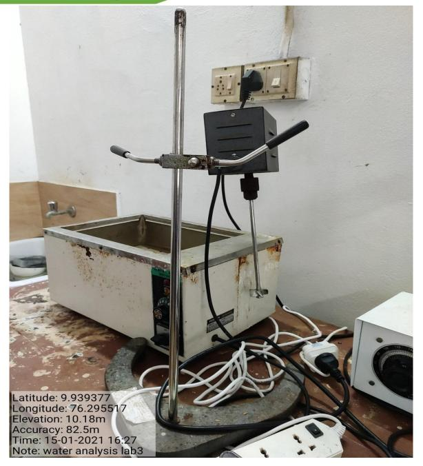
Water bath is a rectangular container including a heating coil at the bottom. It is filled with the water before use. We can adjust the temperature and can be used to keep a reaction for a long time at constant temperature. Once it is put up, the heating coil maintains the constant temperature of water. It can be used for melting of samples and heating of flammable chemicals without the direct explosion to the open flame.
