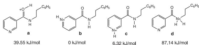
**Scheme 3.** The possible structures of  $[M+H]^+$  ions of compound 1 and their DFT-calculated energies relative to the lowest energy structure (b), at the B3LYP/6-31G(d, p) level.
