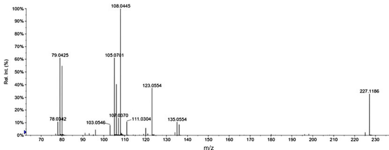
Figure 1. High-resolution ESI-CID mass spectrum of the  $[M+H]^+$  ion of *N*-[nicotinoyl]-2-phenylethylamine.
