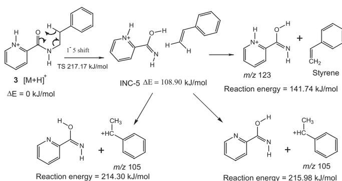
**Scheme 8.** Proposed mechanism of fragmentation of  $[M+H]^+$  ions of compound 3.
