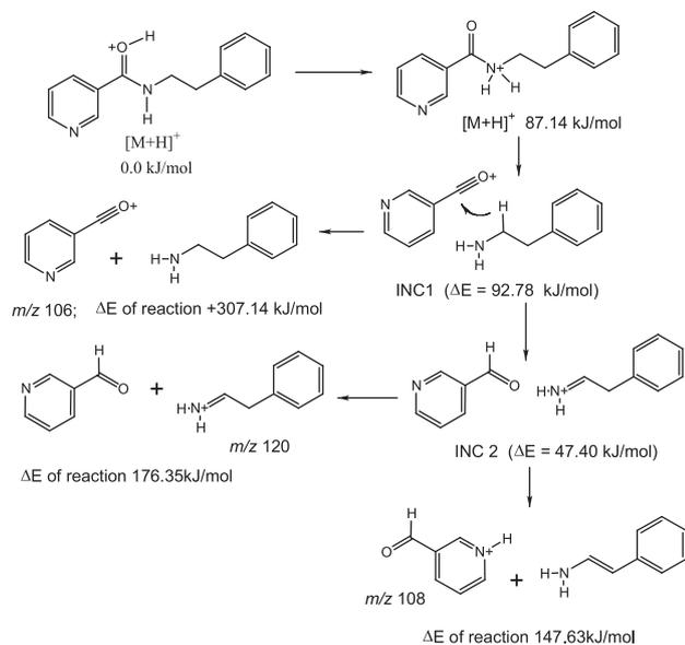
**Scheme 4.** Proposed mechanism of formation of  $m/z$  106, 108 and 120 from the  $[M+H]^+$  ion of compound 1, based on DFT calculations. Reaction energy represents the sum of the energies of cation + neutral relative to that of the  $[M+H]^+$  ion.
