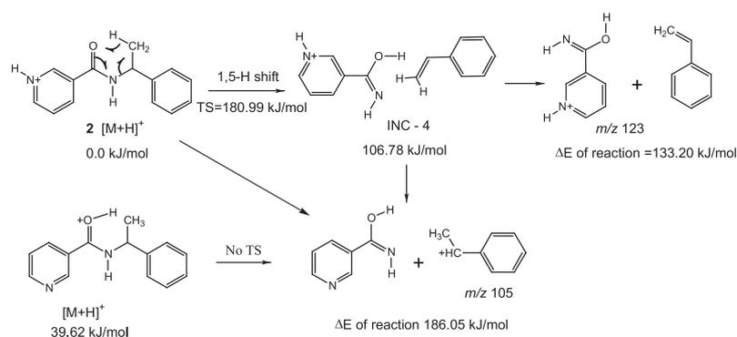
**Scheme 7.** Proposed mechanism of fragmentations of the  $[M+H]^+$  ions of *N*-[nicotinoyl]-1-phenylethylamine (2).
