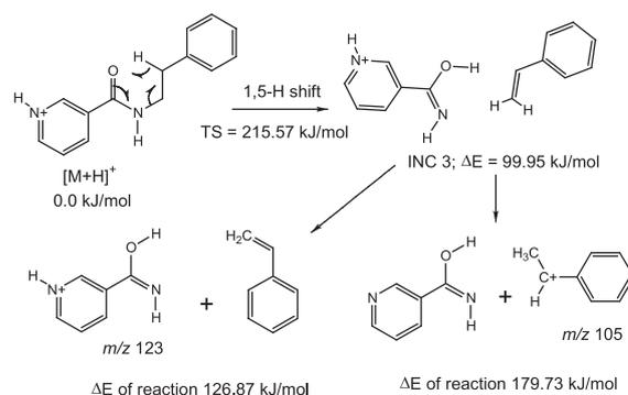
**Scheme 5.** Proposed mechanism of styrene elimination from the  $[M+H]^+$  ion of compound 1, based on DFT calculations. Reaction energy is the sum of the energies of the cation + neutral, relative to that of the  $[M+H]^+$  ion.
