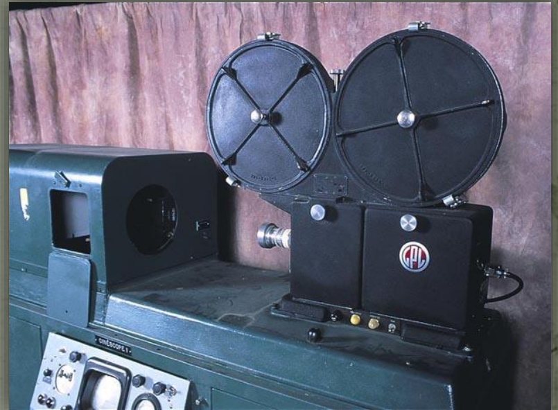
Kinescope recorder recorded images on a video monitor (left) using a film camera (right).
