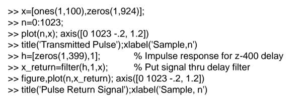
Simulation of a transmitted and received pulse (echo) with a 400 sample delay
