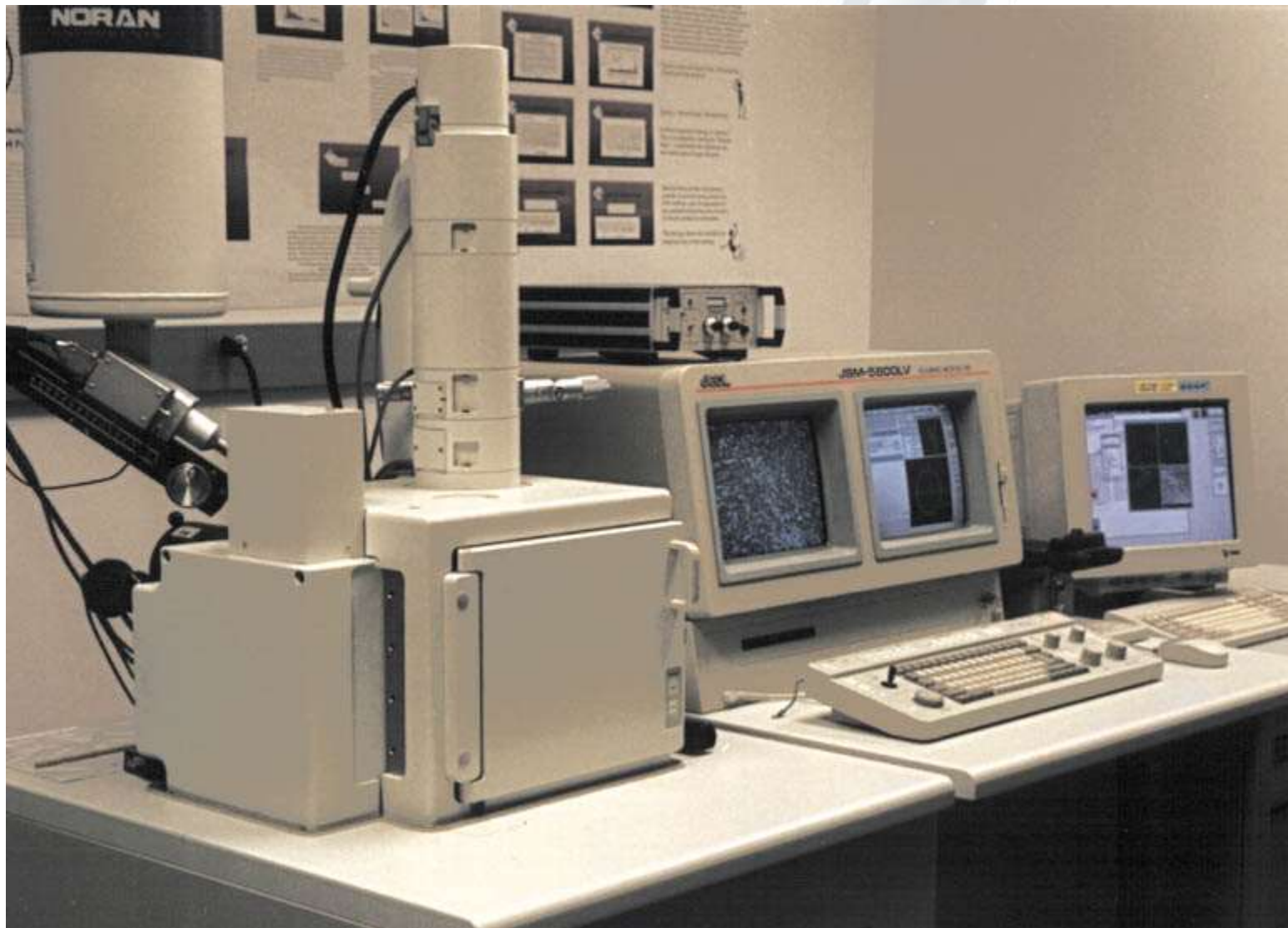
A typical SEM instrument, showing the electron column, sample chamber, EDS detector, electronics console, and visual display monitors.
