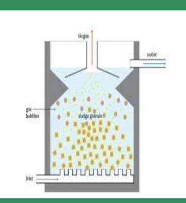
Cross-section of an Upflow <u>Anaerobic</u> <u>Sludge</u> Blanket (<u>UASB</u>) <u>reactor</u>.
