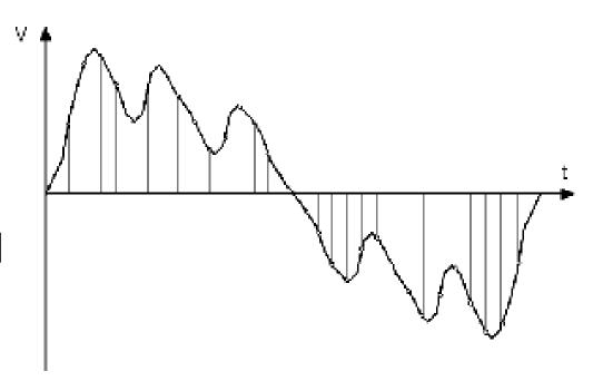
The frequency on which the sampling will occur is called sampling rate. If a sampling rate of 22,050 Hz is used, for example, this means that in one second 22,050 points will be sampled. Thus, the distance of each sampling point will be of 1 / 22,050 second (45.35 μs, in this case). If a sampling rate of 44,100 Hz is used, it means that 44,100 points will be captured per second. In this case the distance of each point will be of 1 / 44,100 second or 22.675 μs. And so on.
