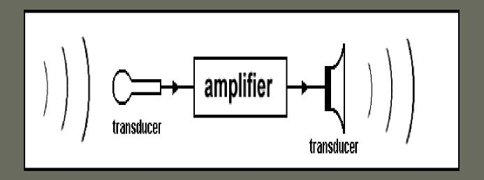
Transducer - A device which converts energy from one form into another. The two types of transducers we will deal with are microphones (which convert acoustical energy into electrical energy) and speakers (which convert electrical energy into acoustical energy). • **Amplifier** - A device which takes a signal and increases it's power (i.e. it increases the amplitude).
