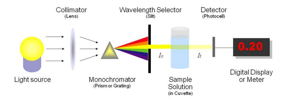
A spectrophotometer can also be designed to measure the diffusivity on any of the listed light ranges that usually cover around 200 nm
