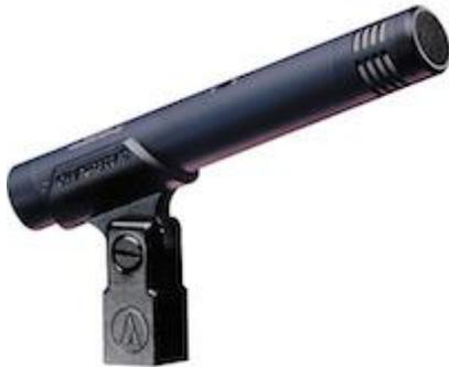
Mics with small diaphragms are commonly called pencil mics because of their thin cylindrical shapes. Their compact design makes them lighter and easier to position, and interestingly, they are designed to be stiffer, to handle higher sound pressure levels and have wider dynamic range. You can use them on acoustic guitars, hi-hats, cymbals, and other instruments. Known limitations of this particular diaphragm type are increased internal noise, and low sensitivity.
