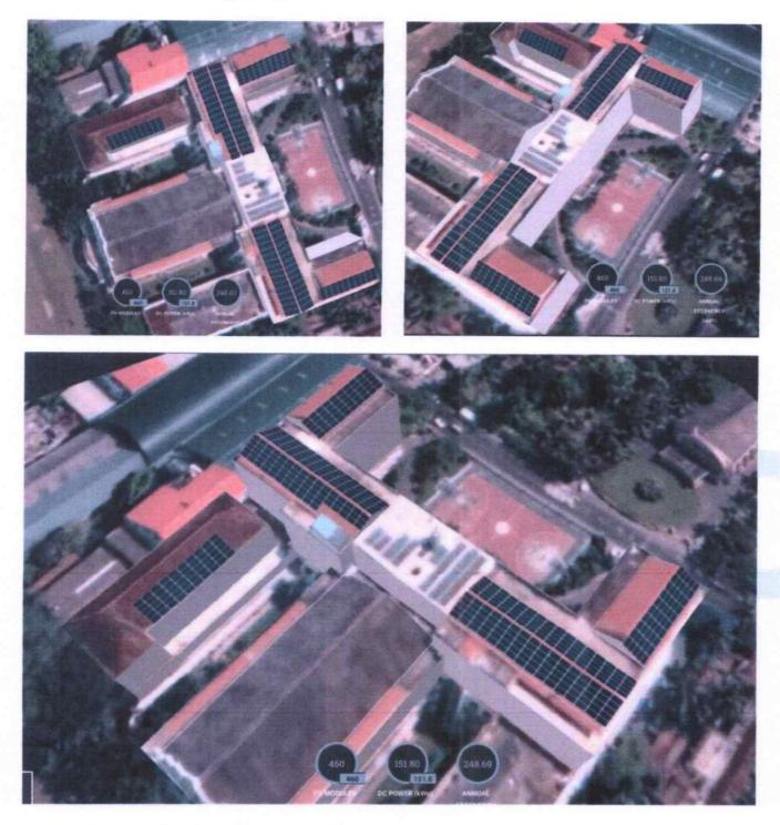
A total of 460 modules of 2m x 1m can be fixed on the current roofs excluding the asbestos roofs of the auditorium. So in short we have more than sufficient area available for generating the entire power required for the college even after accounting for future requirement.
