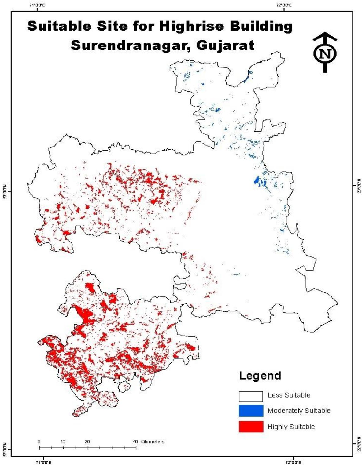
**Fig 4.9: Suitability Map for Highrise building using Model building**
