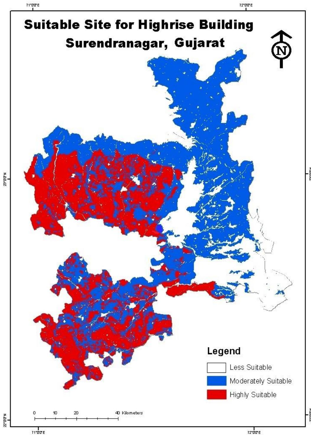
**Fig 4.6: Suitability Map for Highrise building using AHP**
